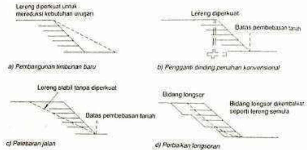
Gambar 2.7 Aplikasi Lereng Tanah Bertulang ( Reifored Soil Slope, Rss )
